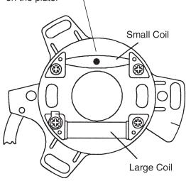
**NOTE:** Black dot on top of small coil will be facing up when the coil is installed on the plate.
