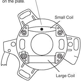
**NOTE:** Black dot on top of small coil will be facing up when the coil is installed on the plate.
