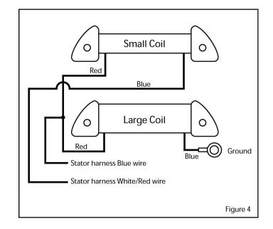
If your stock KDX coils are wired like the diagram in figure 3, wire the Ricky Stator coils as shown in figure 4.
