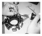
Secure the wires to the stator with a zip tie and reinstall the stator back on to the stator plate. The installation is complete.
