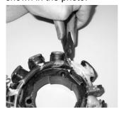
Remove the tape holding the three wires down and separate the wires.
