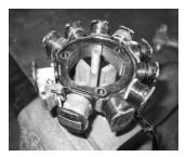
Using a punch, drive the old bobbins out. Note where the big and small bobbins are located.
