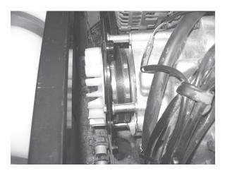
8 Reinstall air shroud cylinder (#48) back onto air shroud (#41). *(See photo)*
