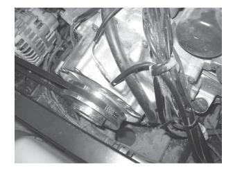
6 Install air shroud (#41) back onto engine using the three provided standoffs and bolts. You will need to drill a hole thru the air shroud (#41) for the top bolt and standoff. This only needs to be done on the top most hole. (See photo)
