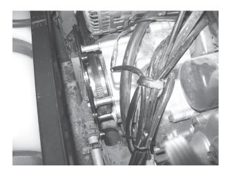
7 Reinstall plate (#47), o-ring (#46), and fan (#43) onto pulley using the bolts provided. (See photo)
