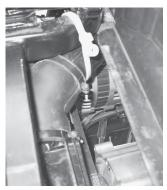
the provided cable ties to secure the duct to the frame ensuring it is not touching the belt. (See photos).
