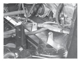
**10** Mount the alternator to the bracket using the two bolts provided. Leave these bolts loose until the final belt adjustment is made. Loop belt over alternator pulley. *(See photo)*
